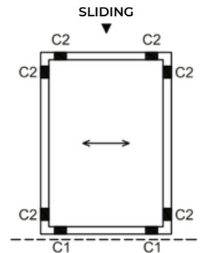
Glazing packers must be placed towards the inside of the bearing points.
